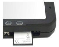
Important: Do Not Insert or Remove the Compact Flash Card while the unit is Powered On.
